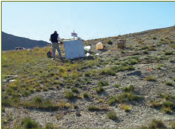
Conducting rainfall simulation to measure erosion on ski run after repeated attempts at revegetation by applying surface treatments.
