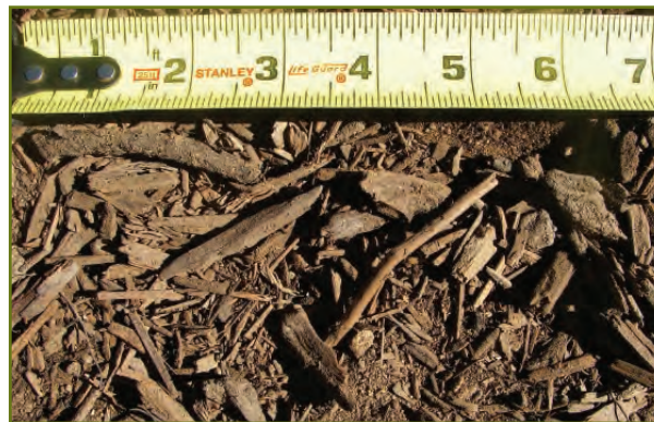
Coarse-textured compost blend – 50% coarse overs (3/8" – 3"), 50% fines (< 3/8")
